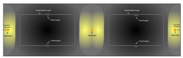
With split feeding systems, install an additional light in the center of the house.
