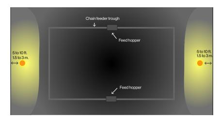
Install Feeding Signal Lights 1.5 to 3 m (5 to 10 ft) from the end wall.
