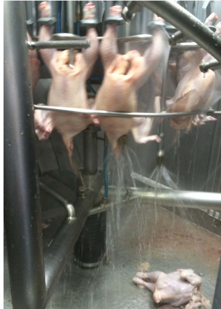
When out of alignment, spray bars to wash probes and contact surfaces can cause product damage or loss.
