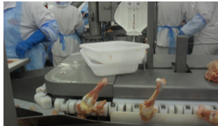
Automated systems are superior to manual system for deboning dark meat based on yield and efficiency.
