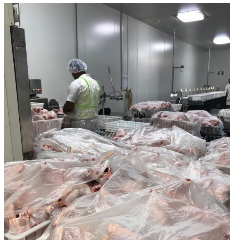
When line speeds after the chiller are slower than slaughter speed, carcasses will accumulate. This can cause yield loss from shrink, process issues from distortions of carcasses and a reduction of shelf-life due to microbiological issues.
