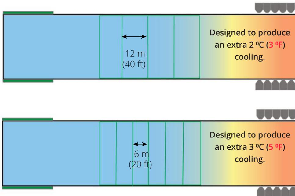
*These are examples of 3 possible configurations that can be used in tunnel ventilated houses. The dimensions and nozzle amounts are approximations. The amount of cooling generated will depend on the water volume generated by the fogger nozzle, water droplet size, dry bulb temperature and relative humidity. The more nozzles the more cooling. Consult your equipment supplier for more detailed information.*
