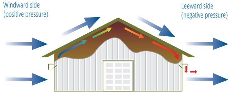
Wind will always create a negative pressure outside on the leeward side, and a positive outside pressure on the windward side. Wind proofing and well-sealed inlets are essential to prevent heat being drawn out of the leeward side of the house.
