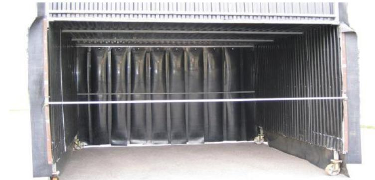
To maximize bird calmness during catching, install portable door curtains to minimize sunlight in the house.
