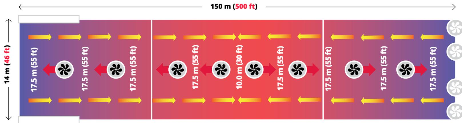
*The large red arrows indicate high velocity movement at ceiling level, while the smaller yellow / orange arrows indicate the low velocity return created at floor level. Increasing circulation fan capacity will increase the “return” air movement at floor level. As long as the return is warm, moving warm air does not constitute as a draft! The more circulation capacity, the drier the litter.*
