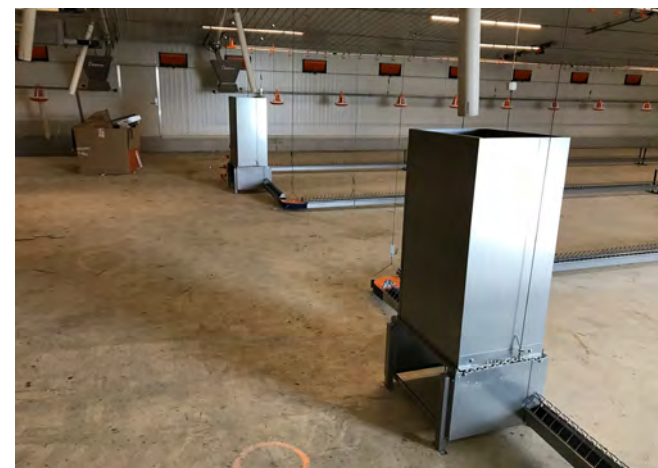
Supplemental hoppers can be added to the system to increase points of feed distribution.
